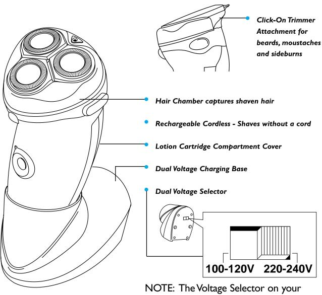
NOTE: The Voltage Selector on your Charging Base makes it possible to charge/recharge the razor on either I10-I20V AC or 220-240V AC. Do not use with Direct Current (DC).
